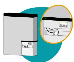
Turn the circuit breaker and auxiliary power disconnect switch to their OFF (0) positions. Wait 5 minutes.
