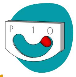
Find the inverter's power toggle switch at the bottom of the inverter module. Turn the switch to the OFF (0) position. Wait 60 seconds.
